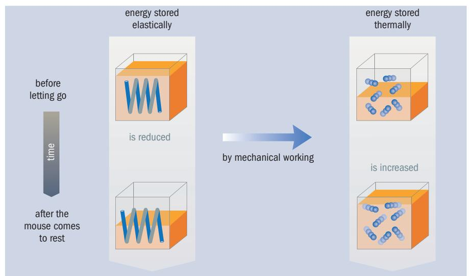
Figure 2. Illustrating how energy is dissipated in the mouse's sprint.
