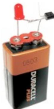
We have constructed an [Electronic Electroscope](#) using a field effect transistor (FET) and an LED. The LED glows brightly when the device is subjected to a positive electric field. This can be used to easily demonstrate the nature of the charge on the Fun Fly Stick and the PVC and cloth. The product is available as "Electroscope & Human Powered Lamp" at [www.profbunsen.com.au](http://www.profbunsen.com.au)
